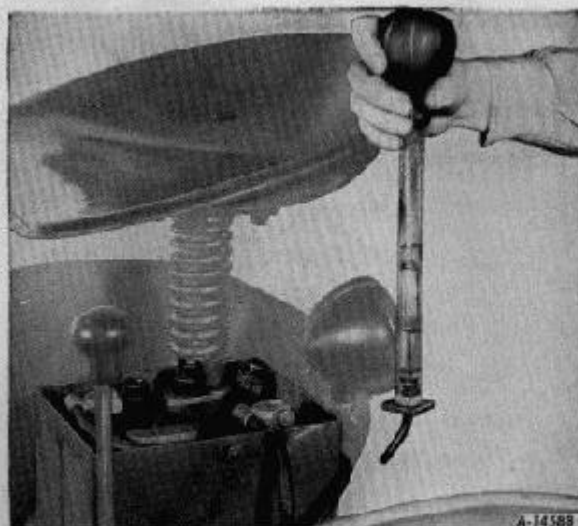
Illust. 71—Taking a Hydrometer Reading of Electrolyte in the Battery.
