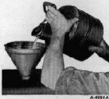
Illust. 8—Filling the Fuel Tank.
